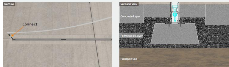
Step 9 ➤ Install the lights and power on.
